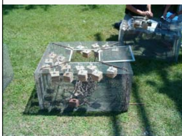
Artificial Substrates (Hester Dendy's) to collect benthic macroinvertebrate tissue.
