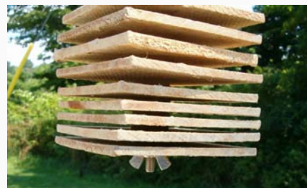
Artificial Substrates (Hester Dendy's) to collect benthic macroinvertebrate tissue.
