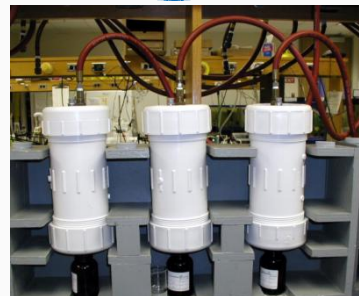
Vacuum Extractor for Pore Water
