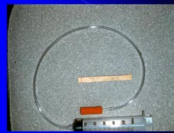
Vacuum Extractor for Pore Water
